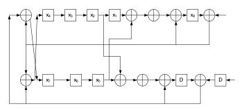
Fig 14.LFSR representation of unfolded architecture for four-level pipelined circuit.
